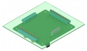
Typical custom PCB: bed of nails test fixture See M&A Board PCB Mount Pattern (last page of data sheet) Separately purchase PCB mount connectors
